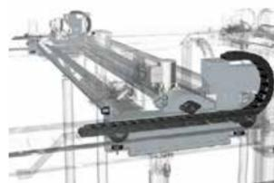
The horizontal brush of the new tunnel is equipped with a travel system that improves the wash of the vehicle rear, with optimum results in the most difficult areas and profiles of the vehicle.
