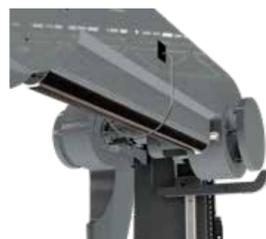
IE3 motors with power levels from 8 to 30 kW add to energy efficiency in the drying step. The horizontal nozzle with its unique three-position design offers an exceptional dry quality with any type of vehicle. 100% textile and non-drip, the Link-dry brush completes the drying process and improves the polish.
