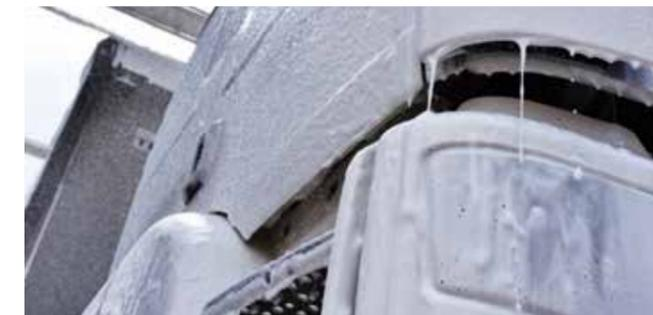
The drive-through chemical pre-wash system applies a more powerful chemical product for fleets needing a thorough clean. Application is controlled by a 100 bar 28 L/min water pump with high chemical resistance and stainless steel pipes. Through a Venturi system, it generates a foamy film that allows the chemical product to work longer over the vehicle surface.
