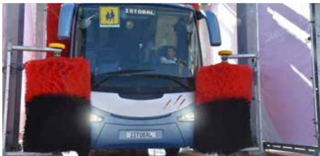
Optional extra for the rocker panel of buses, with brushes with 1.8 metre wash height. Thanks to their small size, they are also capable of washing the front of the vehicle underneath the front mirrors, an area which is usually difficult to reach with the vertical brushes. Controlled by a pneumatic cylinder, these brushes tilt 4°, exerting more pressure on the vehicle's lower areas and tyres.
