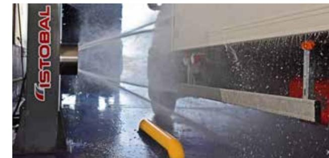
This model offers the possibility of automating the high-pressure process to avoid manually washing the lower sections and the tyres. There are two options: motorised high-pressure lower side rotators that work at 70 bar 84 or 126 L/min, or static side high-pressure with a system of high-impact nozzles located at the bottom working at 70 bar 126L/min. Both options can be installed on the same machine.
