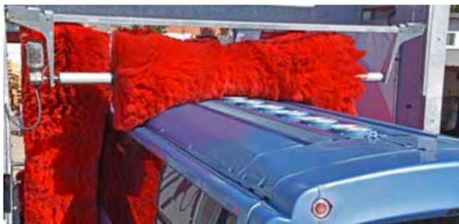
Optional extra for the vehicle roof: it works with a counterweight and a pneumatic cylinder ensuring a smoother operation when the roof surface of the vehicle is washed. With a 1.5 metre travel, it offers a variety of wash heights for fleets with very different vehicle heights. The roof wash contributes to the overall wash result and ensures a higher quality rinse, preventing dirt from the roof from affecting the sides.
