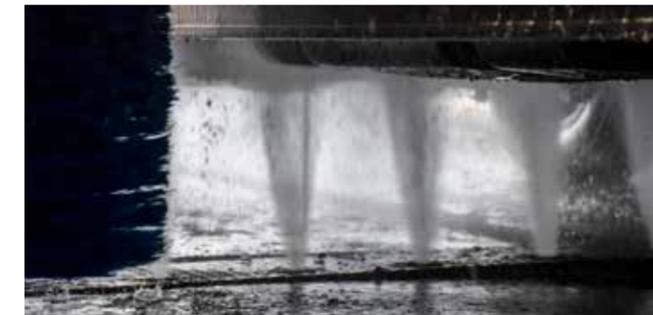
Built into the wash bay and not requiring an independent control system, the underchassis wash works at 70 bar 126 L/min and consists of 10 high-impact nozzles with a 10° orientation towards the vehicle rear to better clean the number plate and the mudguards. It uses the positioning photocell of the vertical brushes, activating the pumps for a limited time and therefore contributing to saving water and energy.
