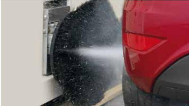
Built-in high-pressure wheel-washer for a thorough wheel-wash, covering the vehicle side as well as the rocker panel. Two-direction spin for a better result on new rim designs.
