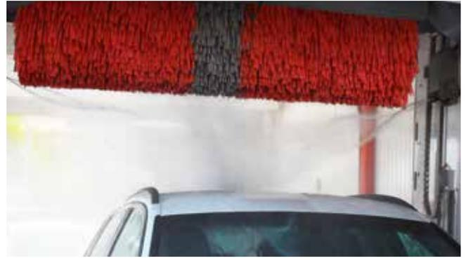
Various high-pressure pre-wash options prepare the vehicle for a subsequent brush wash, optimising the results. Options available from 15 to 160 bar:
